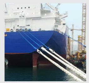
Creep would be a factor in permanent applications such as mooring for long periods of time or guy-wire installation such as for antenna towers
