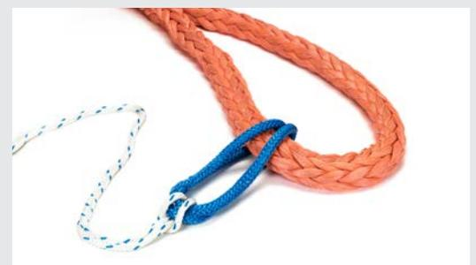
FIGURE 2 A grommet is folded over the eye and the messenger line is girth-hitched to the grommet
