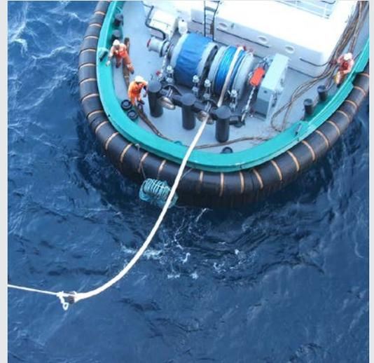
*Use of a multi-directional swivel and recommended messenger line connection method will reduce damage to the pendant eye often seen with traditional connections.*
