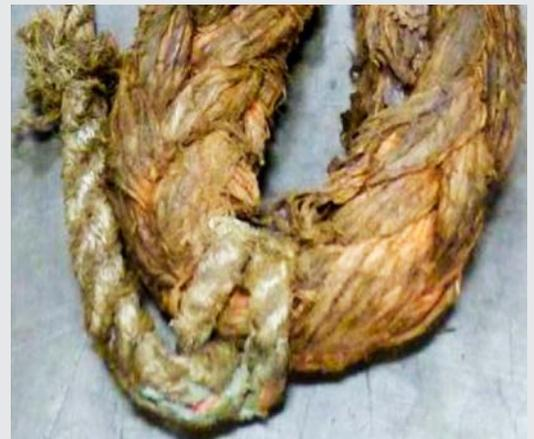
*Typical messenger line girth-hitch connections can cause excessive pressure on the eye when under load, causing internal abrasion and fiber fusing.*
