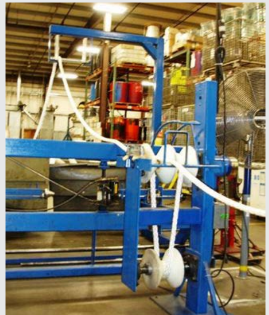
A rope is run over an elevated roller, or through two horizontal breaker bars that add back-tension to control the rope as it is pulled through the reeling system. The rope is then looped around a number of capstans that are controlled to a tension of 10 lb. The rope finally passes through a length counter as it is wound on to the final reel and cut at the required length. The back-tension on the rope as it moves through the counter assists in providing a consistent length measurement and a solidly wound reel.
