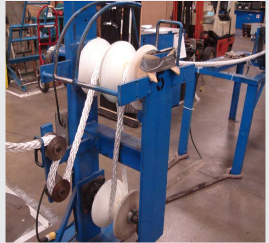
Controlled tensioning system.
