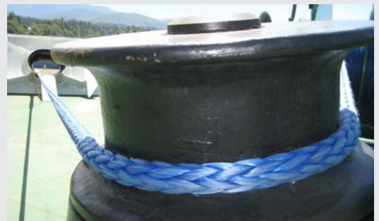
Once contact surfaces have been prepared for HMPE lines continued use of steel-wire ropes is not recommended.
