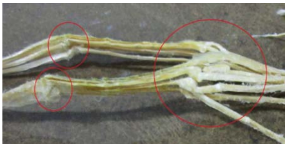
FIGURE 3 Yarn kinks visible to the naked eye in a yarn taken from a jacketed rope
