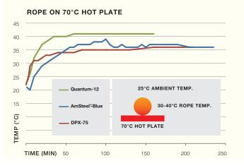
Lab tests placing the ropes on a 70°C constant heat source show the temperature increases with time, as shown in Figure 2. Unsurprisingly, the rope's opposite surface never reaches the heat source temperature, instead reaching a steady-state equilibrium between the heat source temperature and the environment.
