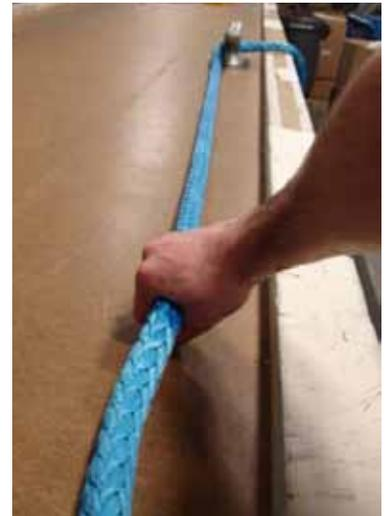
*Tension rope with hand force and measure to reduce the variability in length.*
