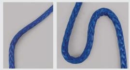
FIGURE 3 Frozen rope bent at  $45^\circ$  on the left and  $180^\circ$  on the right
