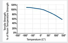
FIGURE 2 Strength of Dyneema® fiber vs. Temperature
