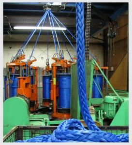
Samson coats the individual filaments in the rope prior to braiding or twisting the final rope to ensure effective coating and limit the potential for static charging.
