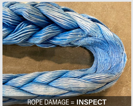
ROPE DAMAGE = INSPECT
