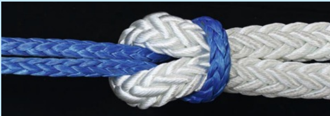
Figure 5.21: Cow hitch connection — HMSF line to polyester tail.
