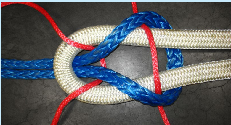
Figure 5.22: Cow hitch connection with pigtail included.
