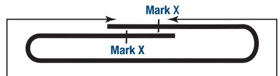
Exact overall lengths with endless loops are determined by allowing for extra rope consumed in making the End-for-End Splice. The length of extra rope is equal to 4 fid lengths.
