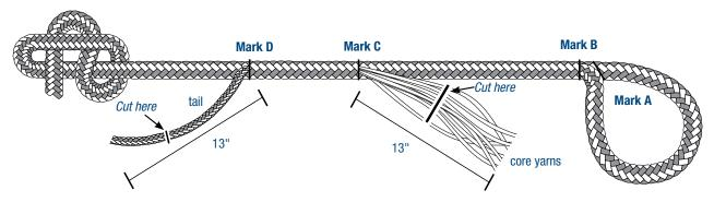
Measure from the cut ends back 6-1/2 inches towards the tail exit points and mark each of the tails. From the mark measure approximately 1-1/2 inches and cut 1 S-twist and 1 Z-twist strand. Continue measuring 1-1/2 inches down and cutting strands until 1–2 strands are left uncut for each tail. This taper provides a smooth transition from the buried tail of the splice to the core yarns extending down the remainder of the rope.
