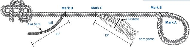
Measure from the cut ends back 6-1/2 inches towards the tail exit points and mark each of the tails. From the mark measure approximately 1-1/2 inches and cut 1 S-twist and 1 Z-twist strand. Continue measuring 1-1/2 inches down and cutting strands until 1-2 strands are left uncut for each tail. This taper provides a smooth transition from the buried tail of the splice to the core yarns extending down the remainder of the rope.
