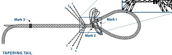
At Mark 3, pull the tail out until Marks 1 and 2 meet. Pull any slack out of the 6 strands that are routed. Pull out the tail and mark 3 consecutive strands as shown. Pull out all 3 and cut.
