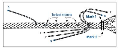
Do 5 complete tucks for all 6 strands. Each strand is always tucked under the same line of the braid so that the tucks progress straight down the body of the rope.
