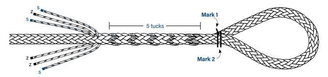
After completing the first 5 tucks, remove 1/2 of the volume of the twisted yarns. Cut yarns from each of the 6 strands near the taped ends and complete 3 more tucks with the reduced volume strands.
