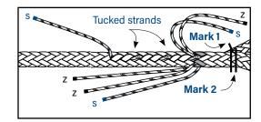
Do 3 complete tucks for all 6 strands. Each strand is always tucked under the same line of the braid so that the tucks progress straight down the body of the rope.
