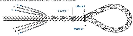
After completing the first 3 tucks, remove 1/2 of the volume of the twisted yarns. Cut yarns from each of the 6 strands near the taped ends and complete 3 more tucks with the reduced volume strands.
