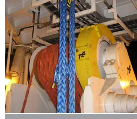
In addition to the buoy pull-in lines, the Stybarrow Venture uses two other high-performance Samson lines: Neutron-8 is installed on the riser-tensioner winches designed by Ram Winch, and AmSteel Blue grommets are used in the riser pull-in system.
