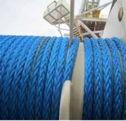
In a typical FPSO mooring application, both wire and synthetic ropes are used on a split-drum winch; however, AmSteel®Blue worked in place of both. The added benefits of its easy handling and change out allowed engineers to simplify the winch-drum design, and provided flexibility overall for the nine-anchor-chain installation and tensioning.
