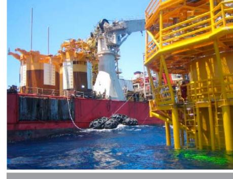
Jeremy White, project engineer for Technip contacted Samson for a solution that would allow the installation to stay on schedule. Samson designed and delivered a set of tapered, jacketed lines with master links spliced into the ends for connection to the riser hoses.
