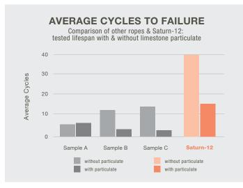
Saturn-12 lasted more than 5 times longer than the average of the other 3 ropes tested.
