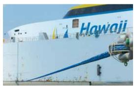
AmSteel<sup>®</sup>Blue holdback lines keep the drydock in position, while the winch lines pull the ferry aboard.
