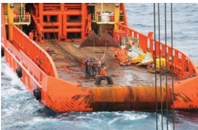
PHOTOS COURTESY OF DELMAR Delmar's OMNI-Max™ anchor is readied for test deployment.
