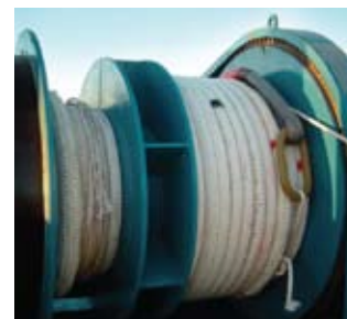
Tapered AmSteel®Blue with polyester jacket winch line, 60-mm diameter tapering to 44-mm diameter with master links spliced in.
