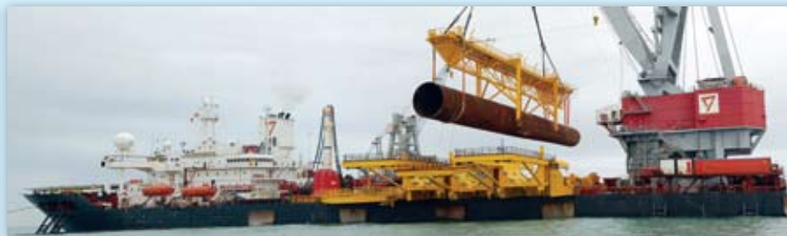
GREATER GABBARD WINDFARM: All 140 turbine foundation monopiles were installed using the first set of lifting slings. After completion Lloyd's proof loaded the slings and recertified them for continued use.
