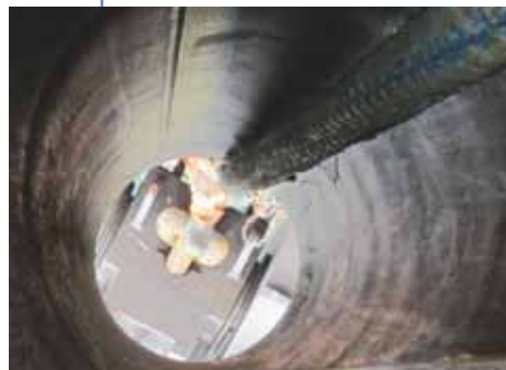
ABOVE AmSteel®Blue brings an anchor chain into its stopper.
