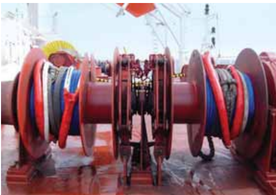
Aft winches, port side, with new AmSteel®-Blue mooring lines installed.
