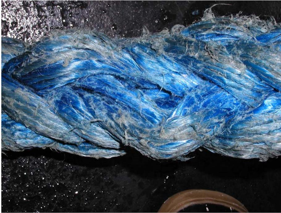
**Figure 5 - Fused yarns, should be inspected further**
