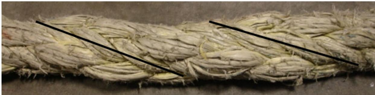
**Figure 10 - Twist imparted in HMPE pendant**
