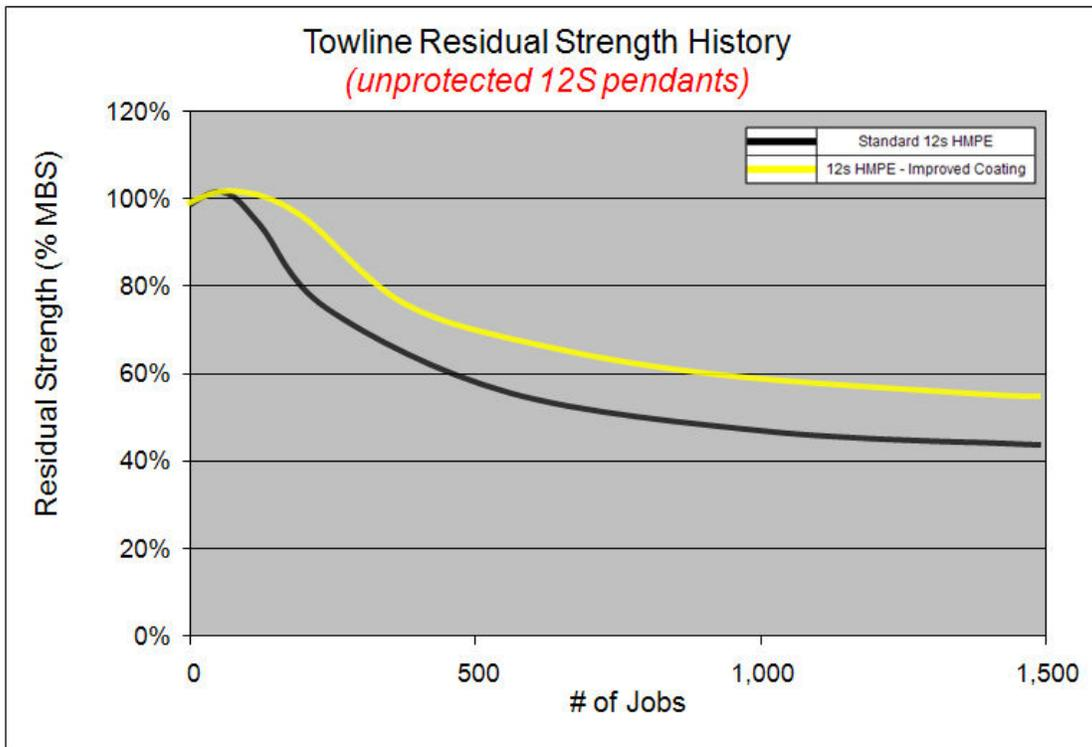
**Figure 6 - Residual strength model comparison**
