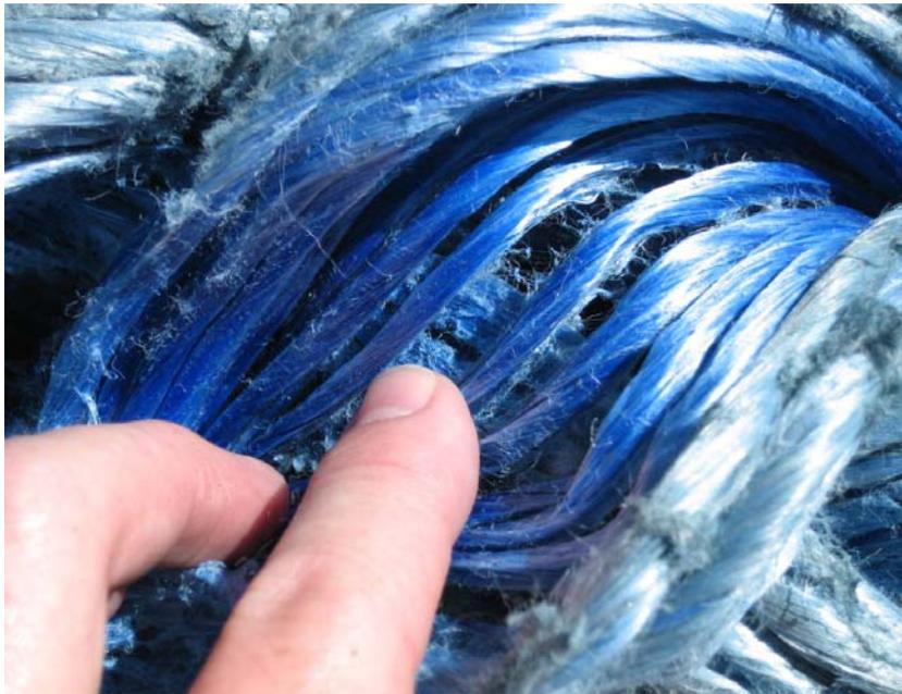
**Figure 7 - Internal wear on standard 12-strand pendant**
