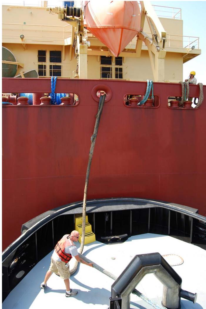
**Figure 1 - Typical Pendant location during ship assist**
