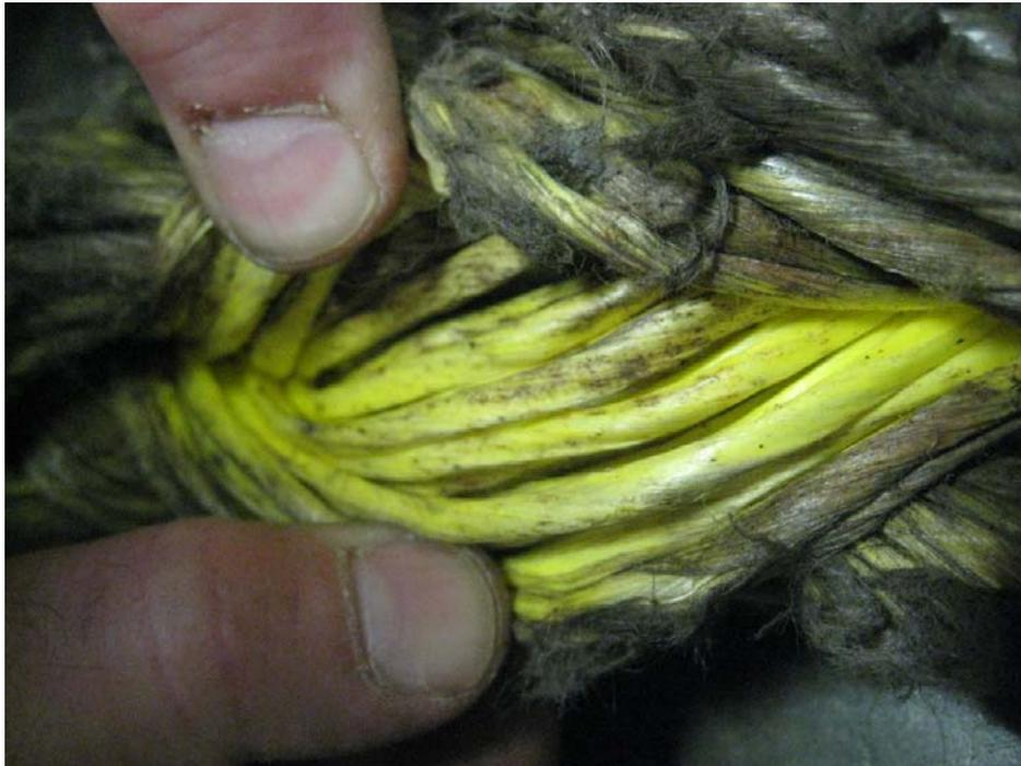
**Figure 8 - Internal wear on 12-strand pendant with improved coating**
