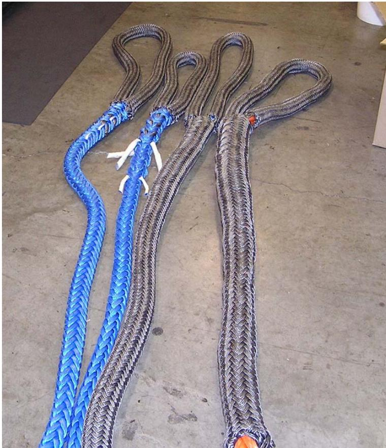
**Figure 2 - Towlines with eye and body braided chafe gear**
