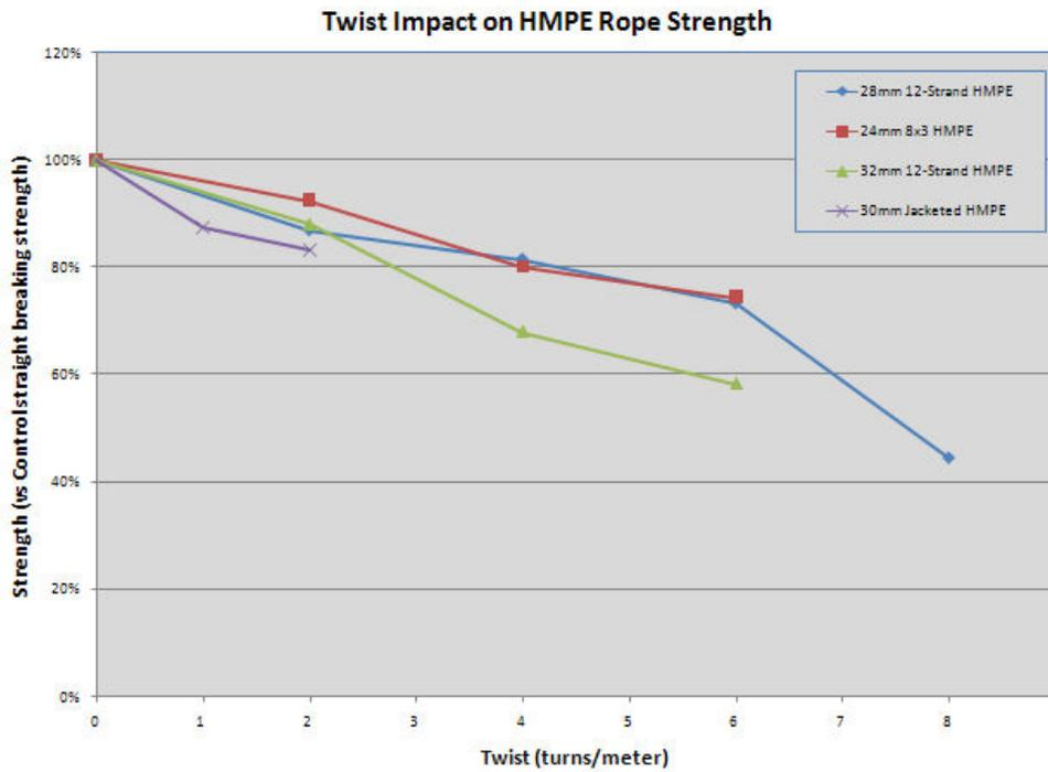
**Figure 9 - Twist impact on HMPE rope strength.**
