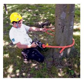
Adjustable lifting slings allow snug lifting control and minimize the number of fixed length slings required.
