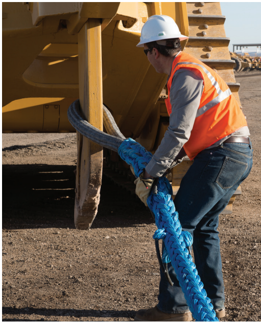
The average time for a change-out is 30 minutes and can be accomplished by one man, dramatically increasing safety and productivity.
